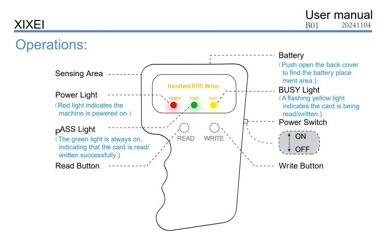
Remove the battery cover and install  $2 * 1.5 \vee$  AAA alkaline batteries. (Note: The device operating DC voltage must be between 2.5 and 3.1V).
